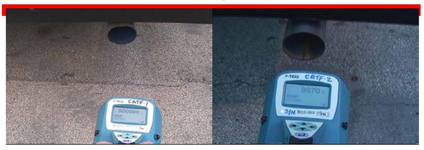
Conventional bus (on left) reads 500,000 ultrafine particles/cc, the upper limit of detection for the PTrak. The bus with a particle trap (on right) reads 9,570 particles/cc—a level that was one third lower than the ambient particle level (~15,000 particles/cc) in Chicago on that day.
